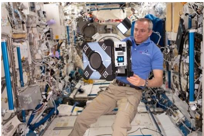
Figure 4. The Astrobeecan free flying robot onboard the ISS.
